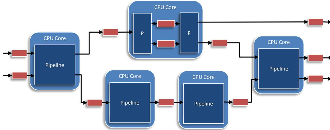
Application is made up of multiple pipelines connected together. Several pipelines can be mapped to the same CPU core.
