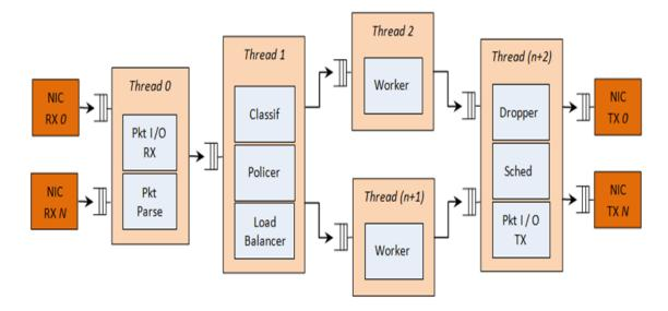
Port/vNIC/ SR-IOV -> UPF - instance / slice , GTP tunnel group per user -> Sub-port , GTP Tunnel (s) ->pipe, Flow -> Queue (WRR/SP)
