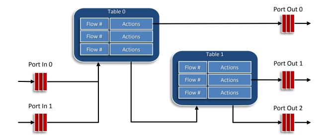
Rapid *pipeline* development out of *ports, tables* and *actions* based on Open Flow inspired methodology
